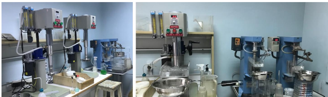
Figure 4. Flotation machines in the experiment to produce gold concentrate
