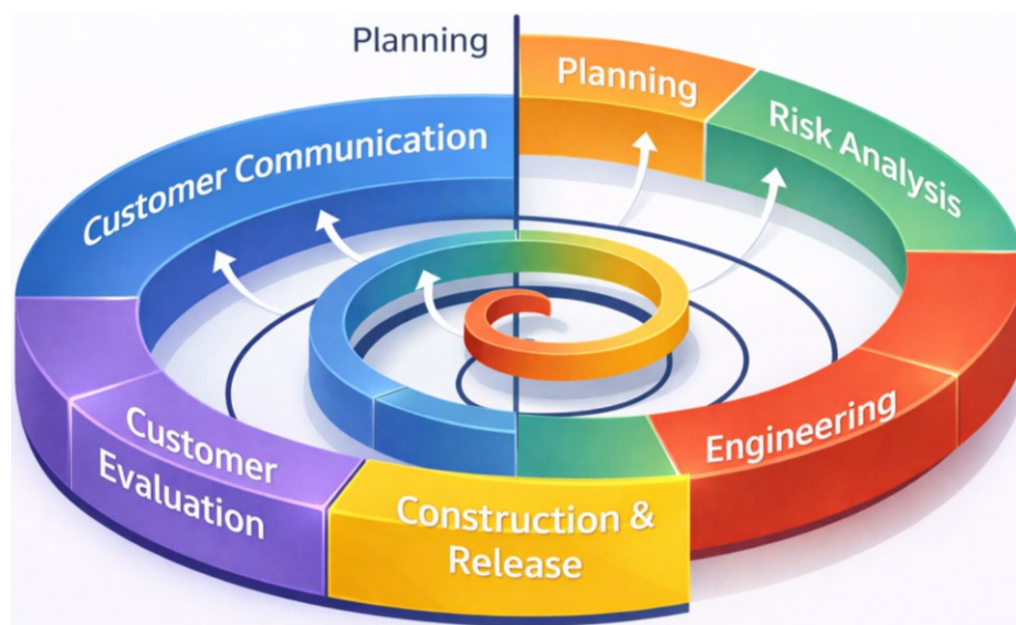
Figure 2. Spiral software development life cycle model
